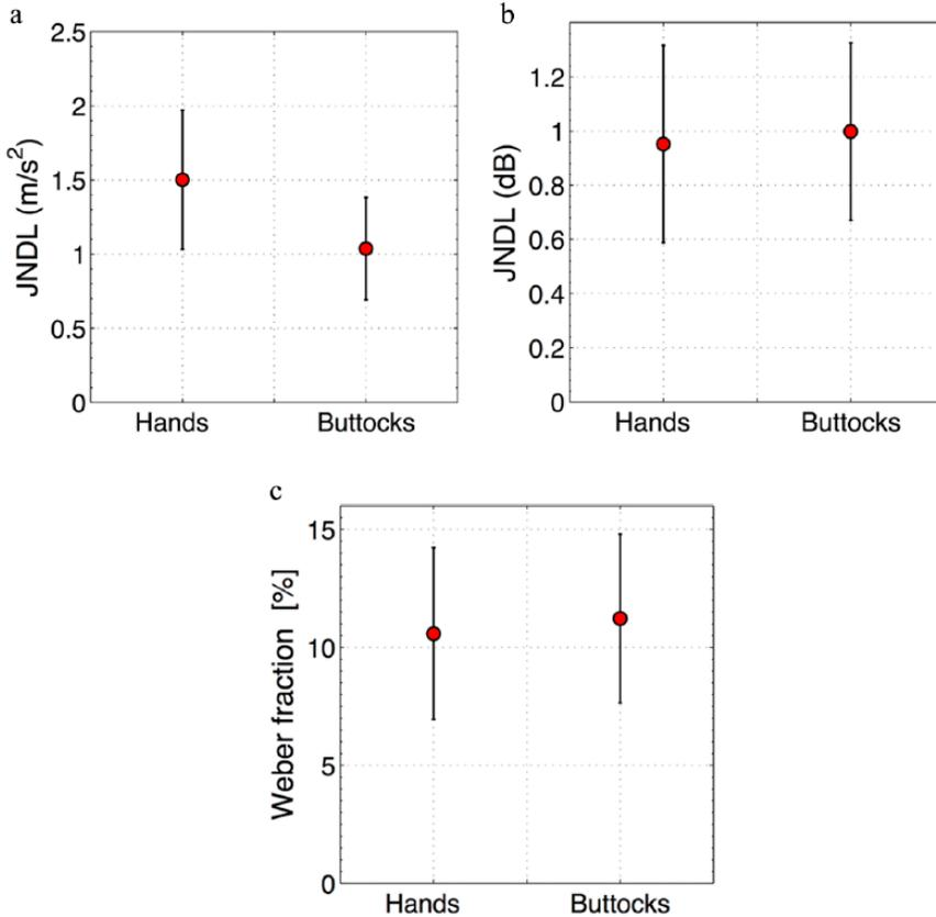
Figure 4. Results of Experiment 1. Mean JNDLs and standard deviations are expressed in terms of acceleration (20 participants). (a) Absolute JNDL expressed in  $m/s^2$ , (b) absolute JNDL expressed in dB, and (c) relative JNDL/Weber fraction expressed in percentage.
