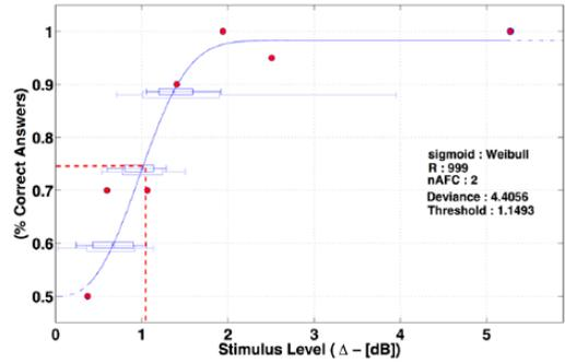
Figure 3. Psychometric curve of a participant estimated using a Weibull function with a 95% confidence interval expressed in dB. The JNDL is estimated as the stimulus level corresponding to 75% correct responses (dotted red line). The error bars represent the estimated variability of parameters, thresholds, and slopes of psychometric functions, obtained from different iteration using bootstrap sampling.
