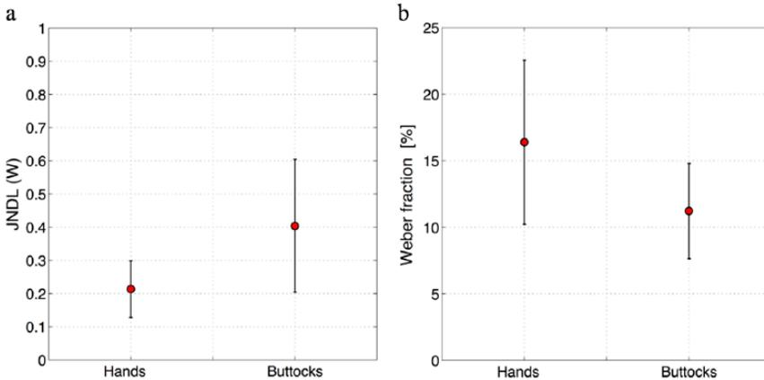
Figure 5. Results of Experiment 1. Average value and standard deviation of the whole-body vibration JNDL using transmitted power (20 participants): (a) absolute JNDL expressed in watts and (b) relative JNDL/Weber fraction expressed in percentages.
