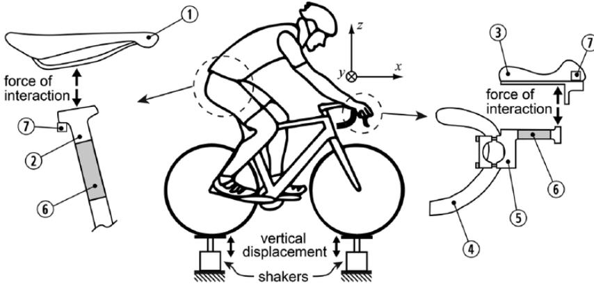
Figure 1. Set-up for Experiment 1: Road simulator was equipped with two shakers for bicycle vibrational transmissibility assessment. The bicycle is equipped with an instrumented seat post and instrumented brake hoods. 1-saddle; 2-seat post; 3-hand rest; 4-handlebar; 5-brake hood body; 6-strain gauges area; 7-accelerometer.
